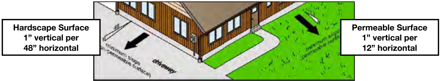
Fig 1 - Drainage Slope Relative To The Structure
