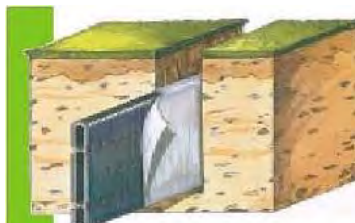
Fig 6 - Interceptor Curtain Drain
